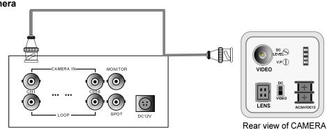
Connect cameras to the camera input on rear panel of DVR marked CAMERA IN.
